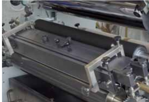
Feeding box for hotmelt coating out of the nip
